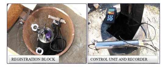
Fig. 3. Automatic measuring system for monitoring groundwater in the well of the state reference observation network
