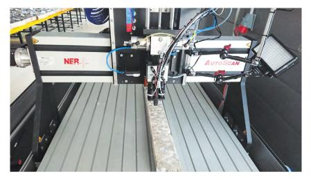
Fig. 6. AutoScan-II integrated measurement platform
