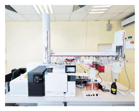
Fig. 5. Agilent GCQTof 7250 high resolution time-of-flight combined gas chromatography mass-spectrometer
