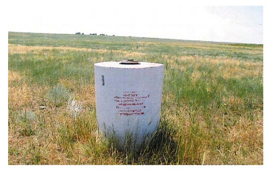
Fig. 2. Well of the state reference monitoring network for groundwater monitoring
