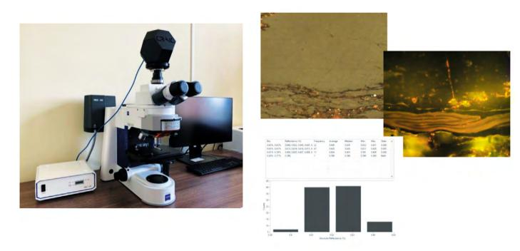
Fig. 3. Axio Imager A2M microscope with CRAIC Coal ProIII.QD1302 (Craic Technologies) photometer adapter and the results of coal petrography investigations
